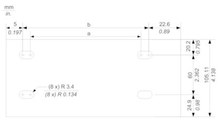
**NOTE:** You can use M4, M5, M6, or UNC #6 screws in the fastening holes. Dimensions in mm
